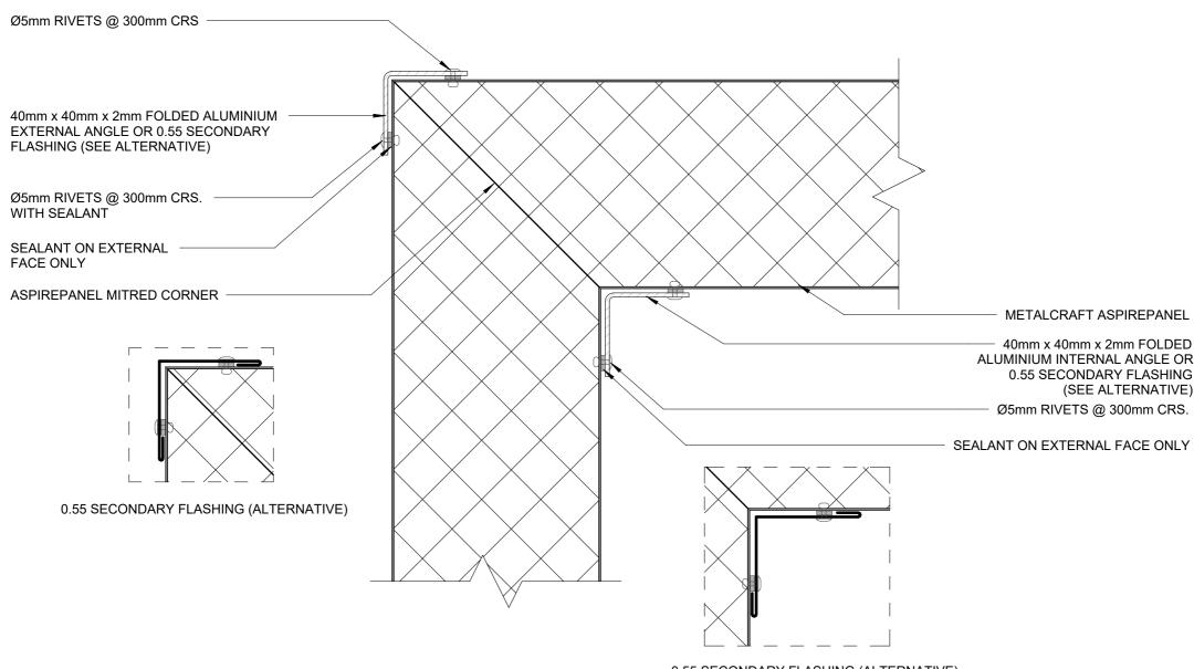
**ALUMINIUM ANGLES CAN BE** REPLACED WITH STEEL
