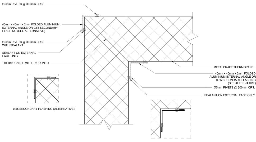
**ALUMINIUM ANGLES CAN BE** REPLACED WITH STEEL
