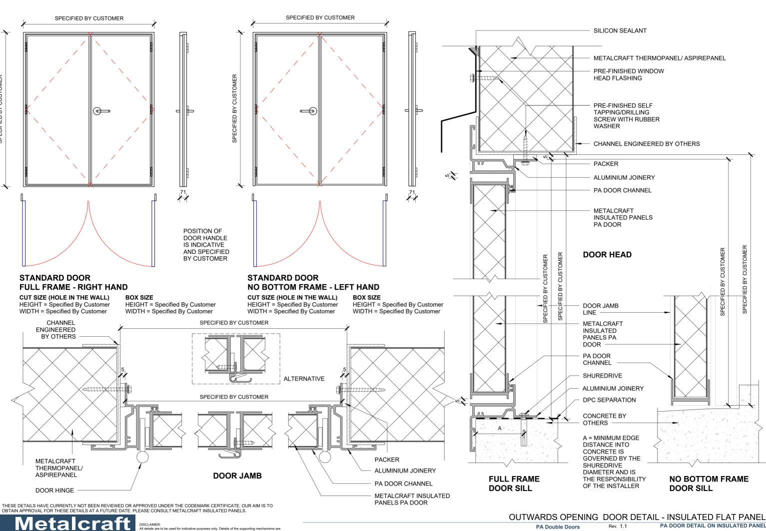
All details are to be used to initiative purposes only. Detains on the supporting frequenties and indicative only and require engineering by others. Compliance of the supporting mechanisms is the responsibility of the designer. Construction detail can vary for wall cladding. The underlay is detailed as a single line for simplicity and is indicative only. Building paper type and method of installation should comply with underlay manufacturers recommendations and NZBC regulations.
